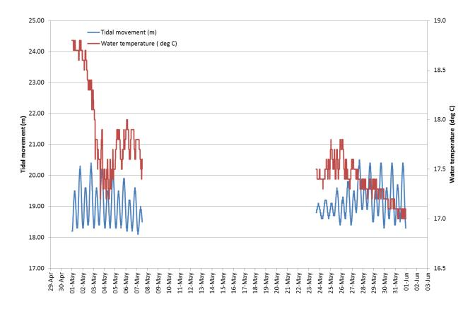
**Figure 5**. Changes in dissolved temperature ( $^{\circ}$ C) with tidal movement (m) over 16 days, 1<sup>st</sup> May to the 7<sup>th</sup> May 2014 and 23<sup>rd</sup> May to 31<sup>st</sup> May 2014.
