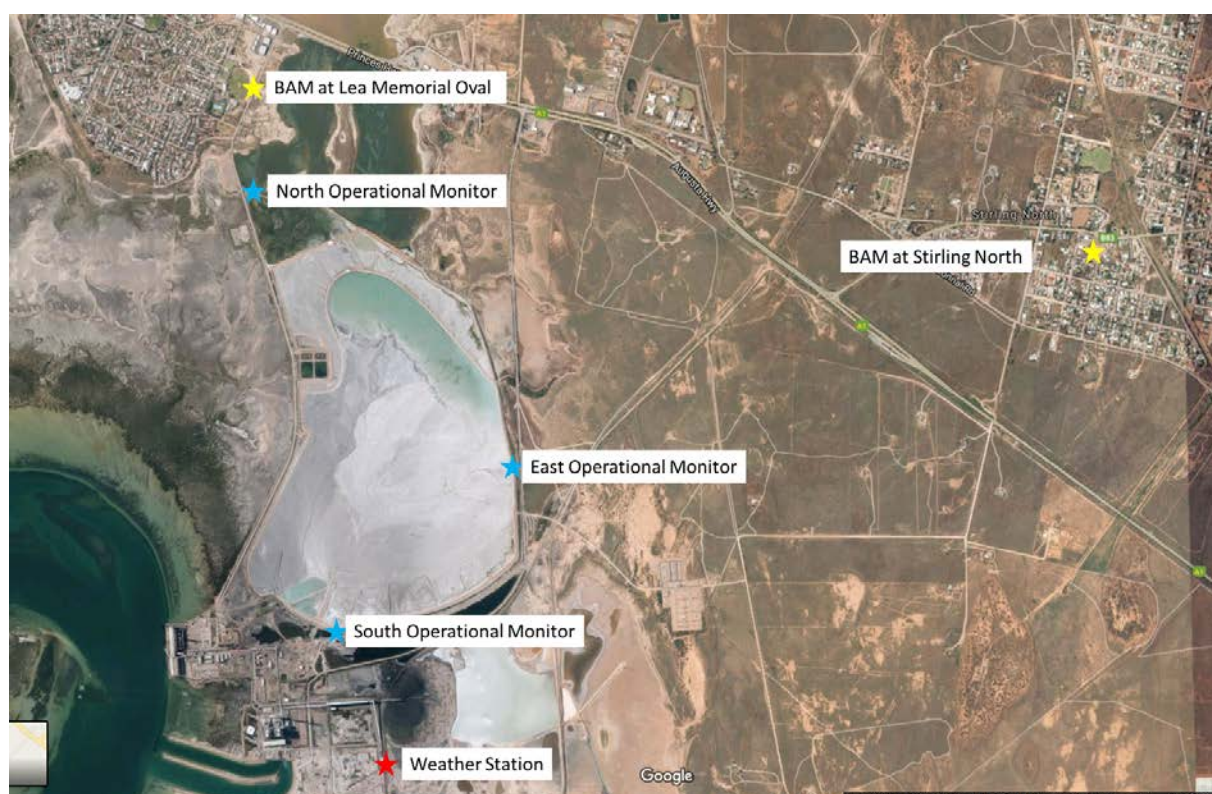
Figure 1 – Real-time Continuous PM10 Dust monitoring locations – Ash Storage Area & BAM Locations
