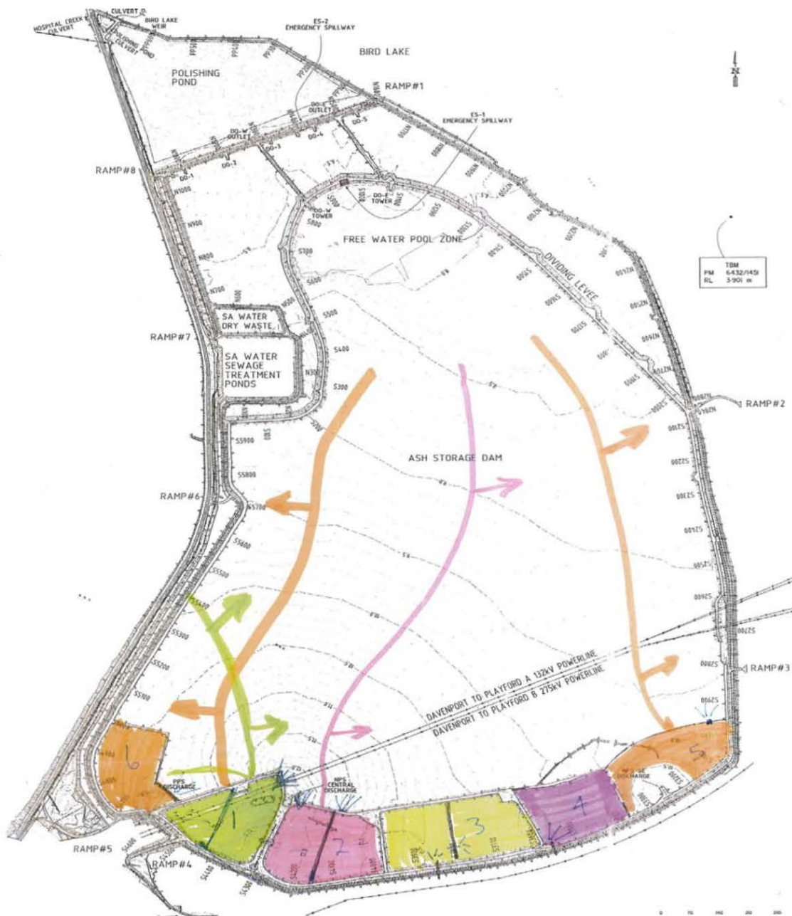
Figure 3 Ash Storage Area map showing numbered flood coffer dams and direction of floodwater flow during surface flooding events.
