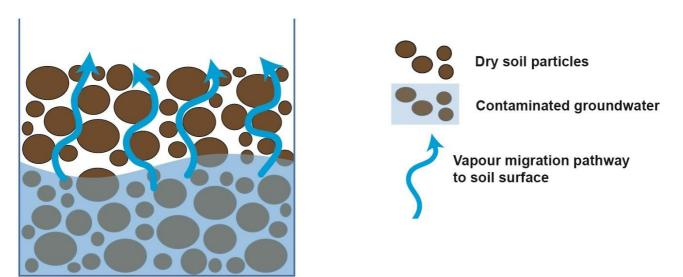
When volatile chemicals such as TCE are present close to residential properties, contaminated vapour can enter homes through small pathways such as cracks in foundations or floorboards. This is called 'vapour intrusion'.
