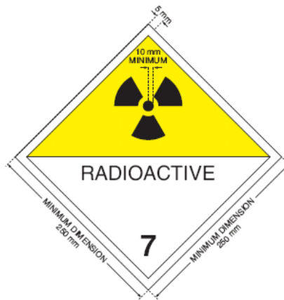
Figure 2 Placard for Radioactive Material
