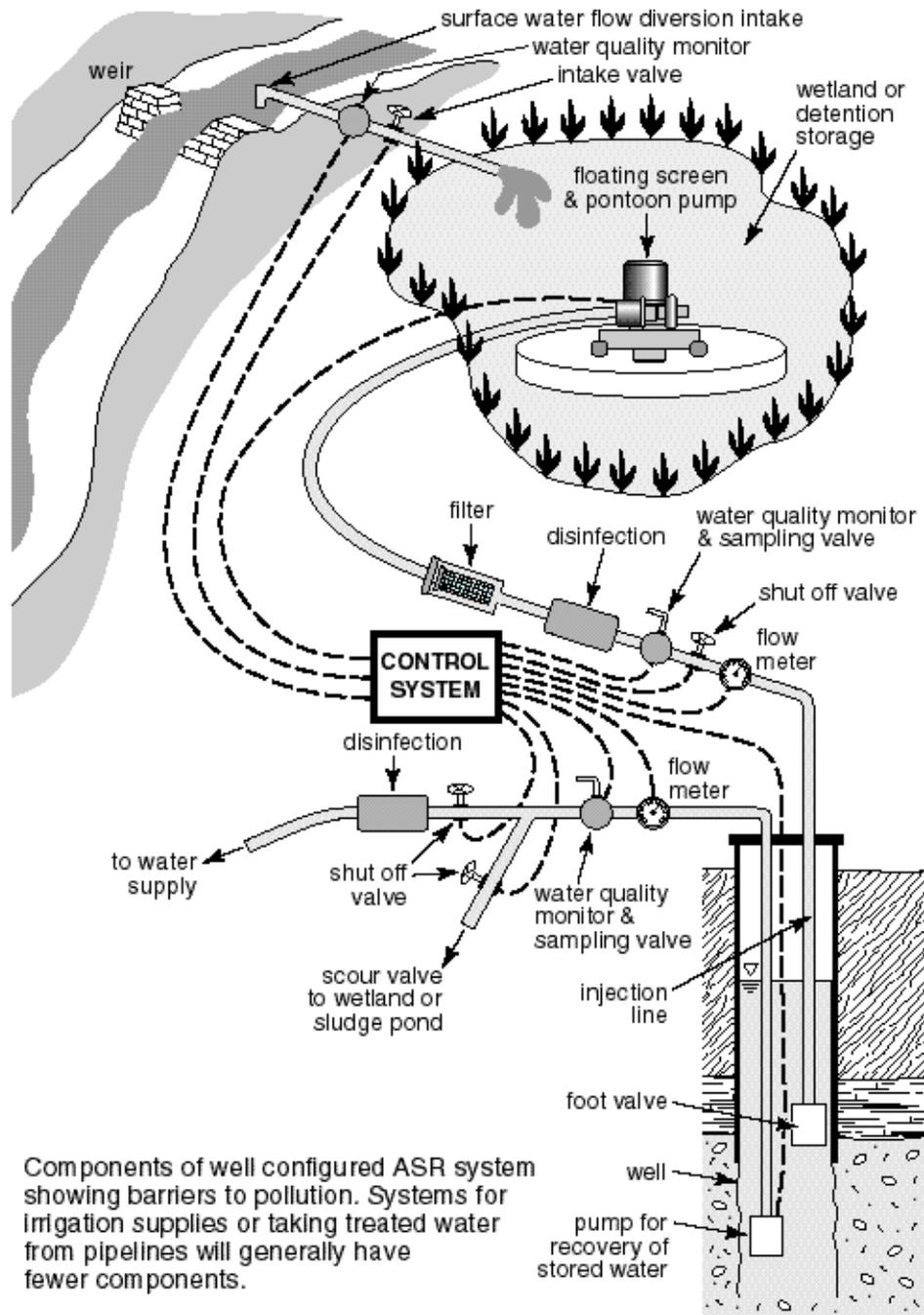
Figure 1 Components of a well-configured ASR system (diagram CSIRO Land & Water)
