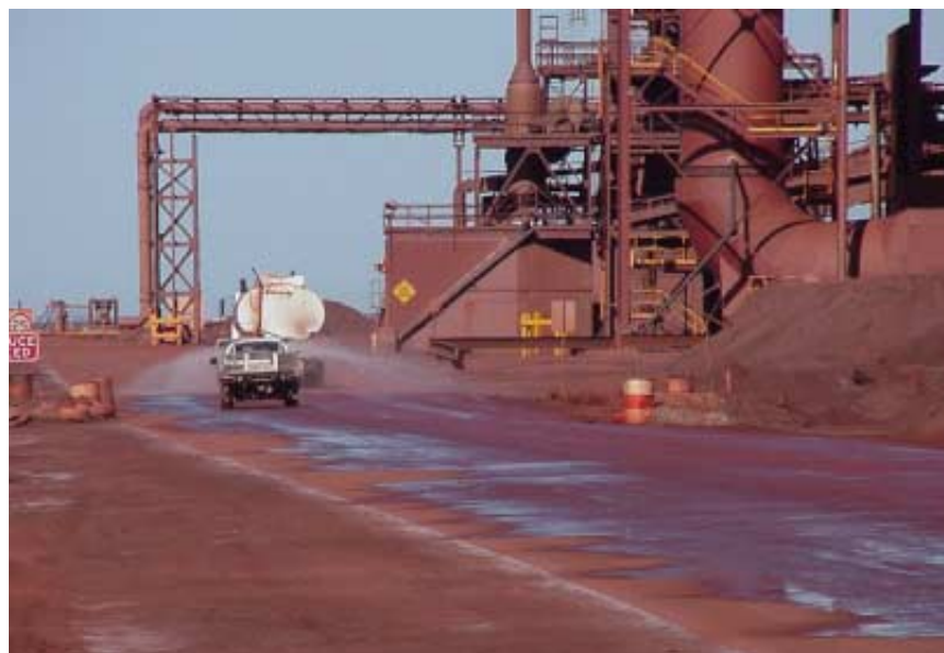
Figure 22. A water truck prevents fugitive particles escaping from roads at the pellet plant (photograph: EPA, August 2001)
