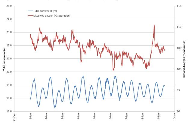
**Figure 2**. Changes in dissolved oxygen (%) with tidal movement (m) over nine days, from  $1^{st}$  January to  $9^{th}$  January 2014.
