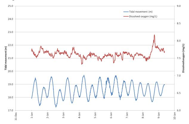
**Figure 3**. Changes in dissolved oxygen (mg/L) with tidal movement (m) over nine days, from  $1^{st}$  January to  $9^{th}$  January 2014.
