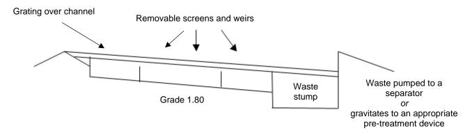
Figure 2. Diagrammatical view of the technical features of a wash down area Source: Industrial Wastes Vehicle Washing Policy, SA Water (1997)
