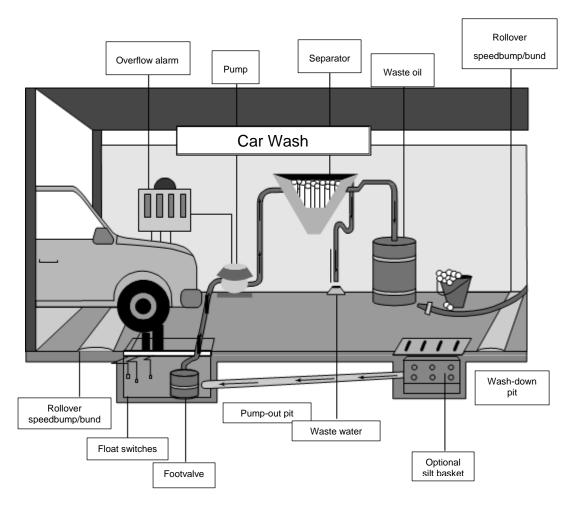
Figure 1. This picture shows the principal features of a well-designed wash bay.
