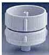
This is a two-piece filter holder that screws together with a filter paper inserted in between the two halves. They are a step down from the filtering unit, as they have no vacuum vessel. The lack of vacuum vessel means that they are difficult to attach to a standard pump, but a large syringe works particularly well.
