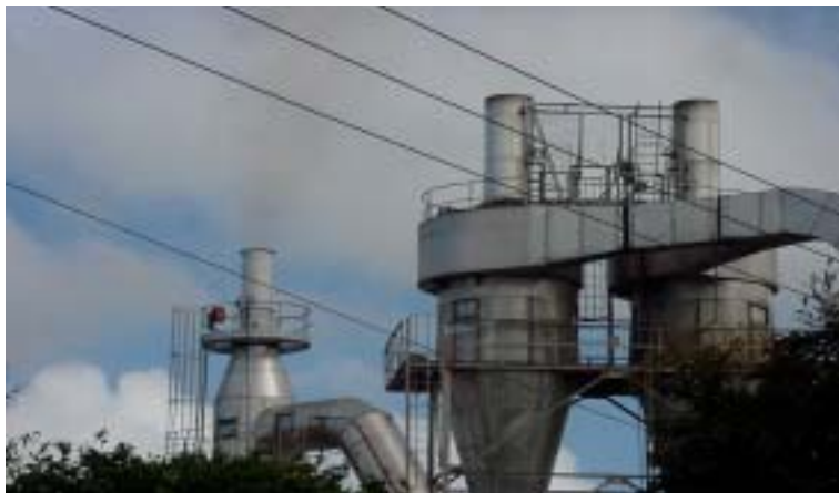
Figure 5 Smokey air emission stacks associated with the wood chip dryers at the Carter Holt Harvey, White Avenue site
