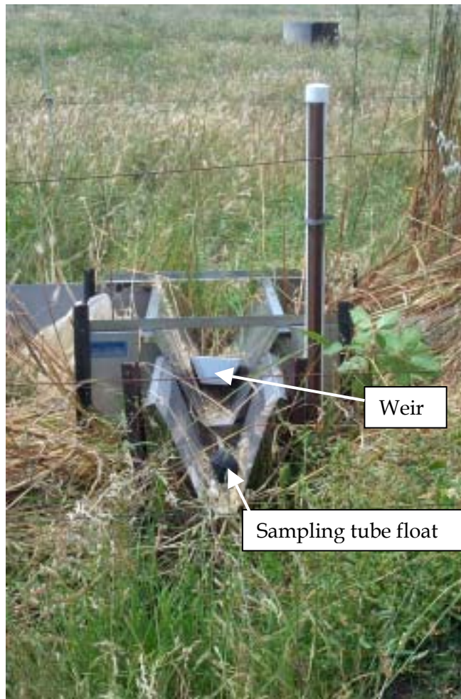
Plate 2 BC 150 flume as installed at the Flaxley sites
