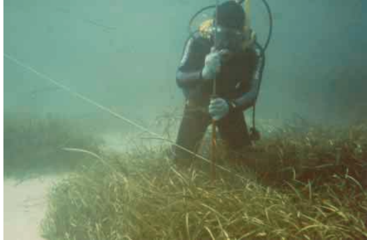
Figure 4 Monitoring sand movement and blowouts with rods (photo: D Fotheringham).
