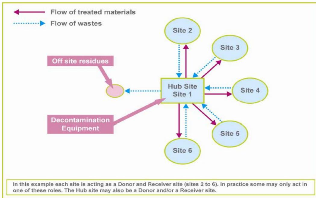
Figure 8 Soil bank operation
