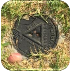
Small caps will be placed over each testing location
