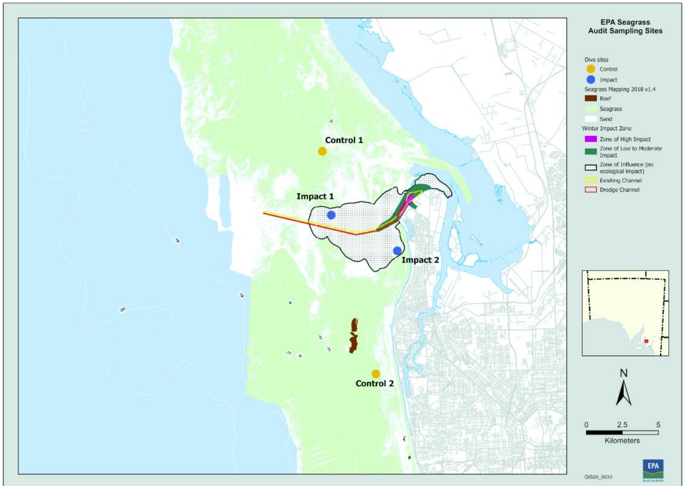
Figure 2 Predicted dredge impact zones from Flinders Ports modelling of the Outer Harbor channel widening project (BMT 2020). Seagrass cover determined by aerial photography overlaid (Clarke et al 2018) with locations of control and impact sites for seagrass condition assessment.
