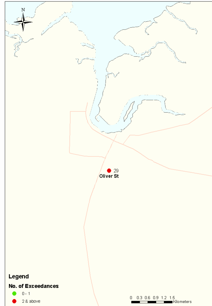
Figure 46 Number of exceedences of the 1-hour sulfur dioxide NEPM standard (0.20 ppm) in the Pt Pirie airshed
