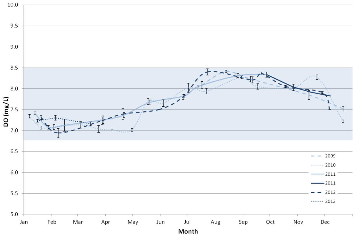
Figure 8 Average dissolved oxygen concentration (mg/L) on the seafloor, 100 metres from the diffuser location at a depth of 15 m to 20 m. Error bars represent standard deviation. Note that the Adelaide Desalination Plant started to discharge saline concentrate intermittently from September 2011 (represented by dark blue lines). The shaded area represents the normal dissolved oxygen concentration in the Port Stanvac region.
