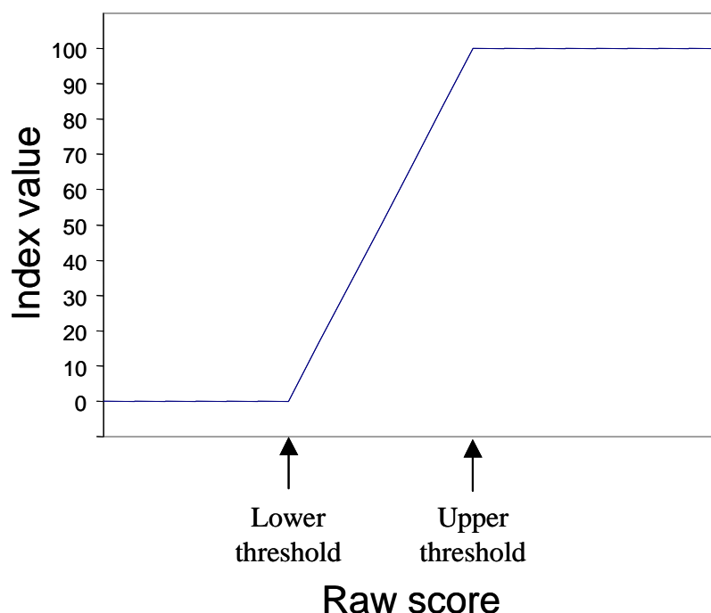
Figure 2. Example scaling of a positive index (a negative index would be the mirror of this plot). Raw figures less than the lower threshold received the minimum value (0), between the two thresholds the index was scaled linearly between the minimum and maximum (100), and for raw scores greater than the upper threshold the maximum index value was recorded.
