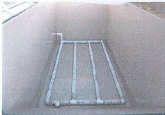
Left: Ventilation pipes placed on bottom of Bio - Composter bin. Right: A layer of Chip is spread over pipes to prevent clogging.
