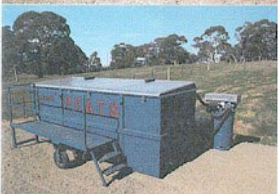
Left: Complete Bio-Composter unit installed and operational. Right: Mortalities are placed in bin, alternating one side to the other.
