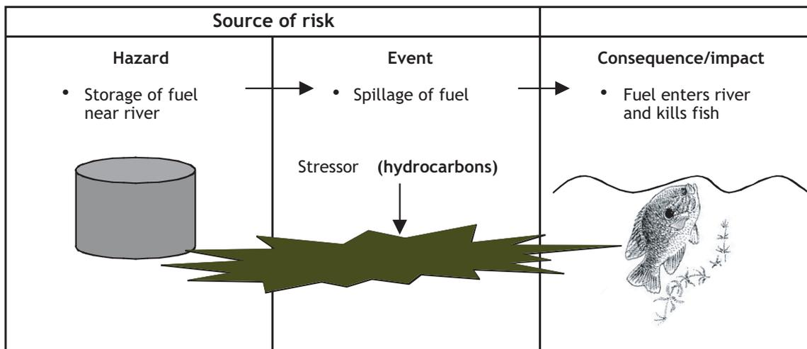
Figure 2.3 Schematic diagram of terminology (adapted from HB203:2004)
