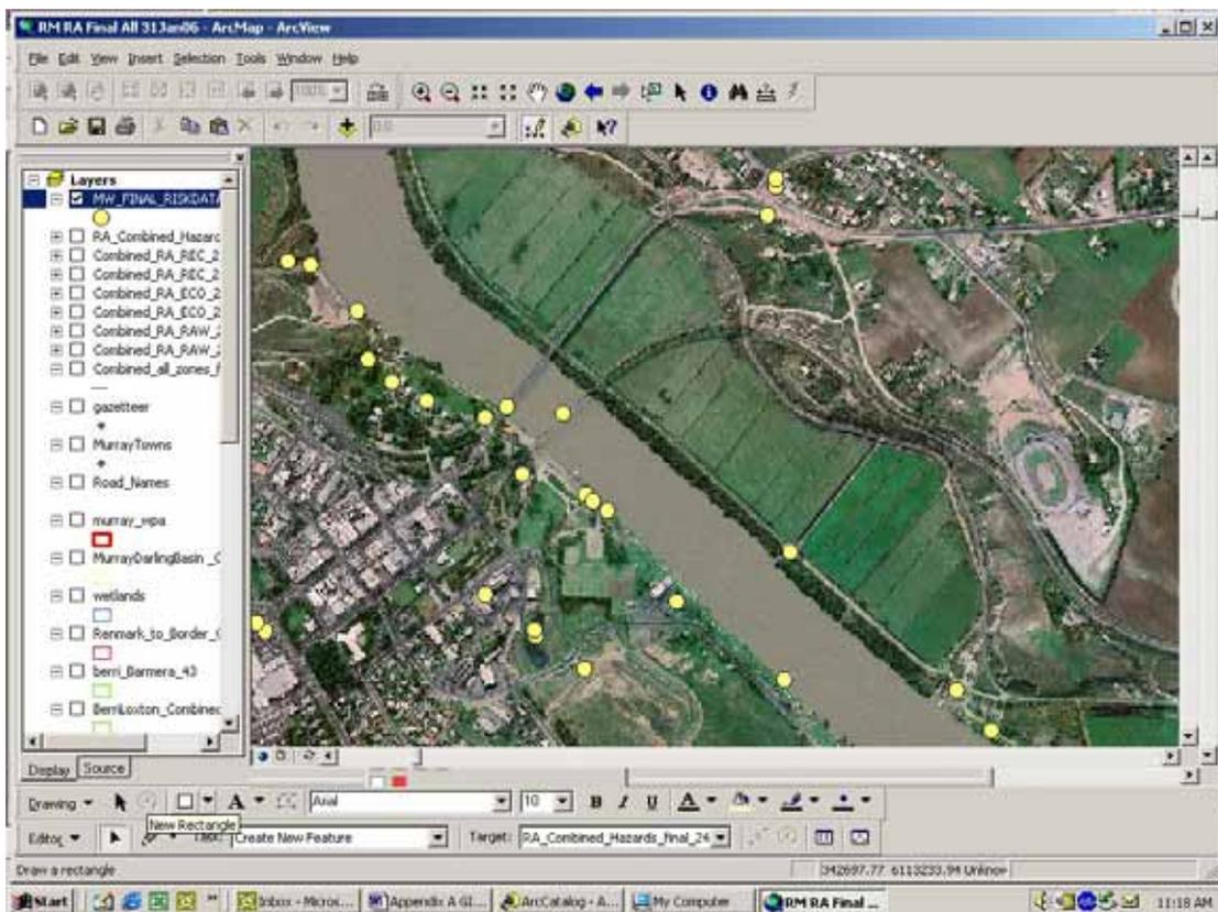
Figure B1 High-resolution aerial photograph with hazard (point) locations (yellow circles)
